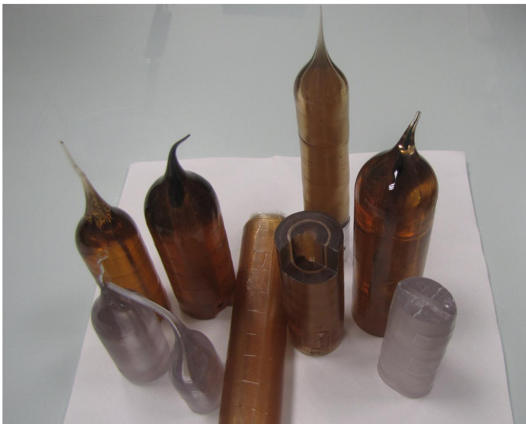
Figure 2.1: Photographs of macroscopic preforms. Preforms are macro prototype of fabricated micro- or nanostructures. The design of preform may change depending on the purpose of fabrication and geometry of nanostructures.
